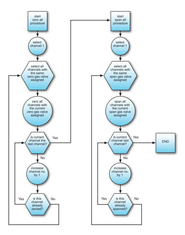
Fig. 7-6: Zero Span All Calibration Procedure Flow Diagram
